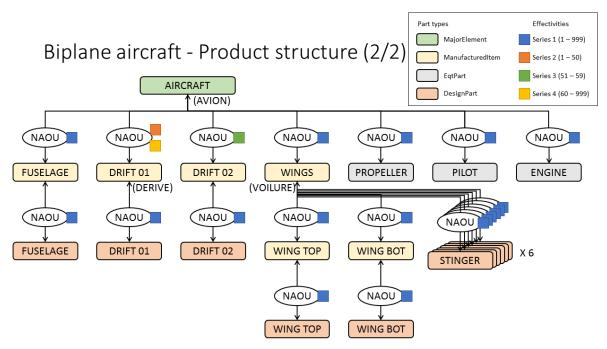
Figure 4: CONF2 Assembly Structure
