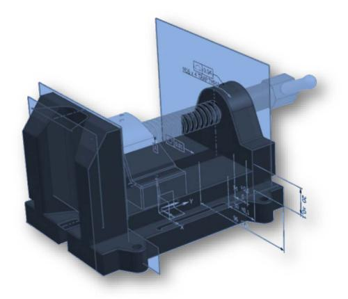
Figure 2: prostep ivip "Vise" Test Model Overview
