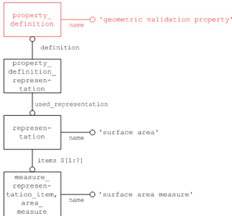
Figure 4: Geometric Validation Property "Surface Area"
