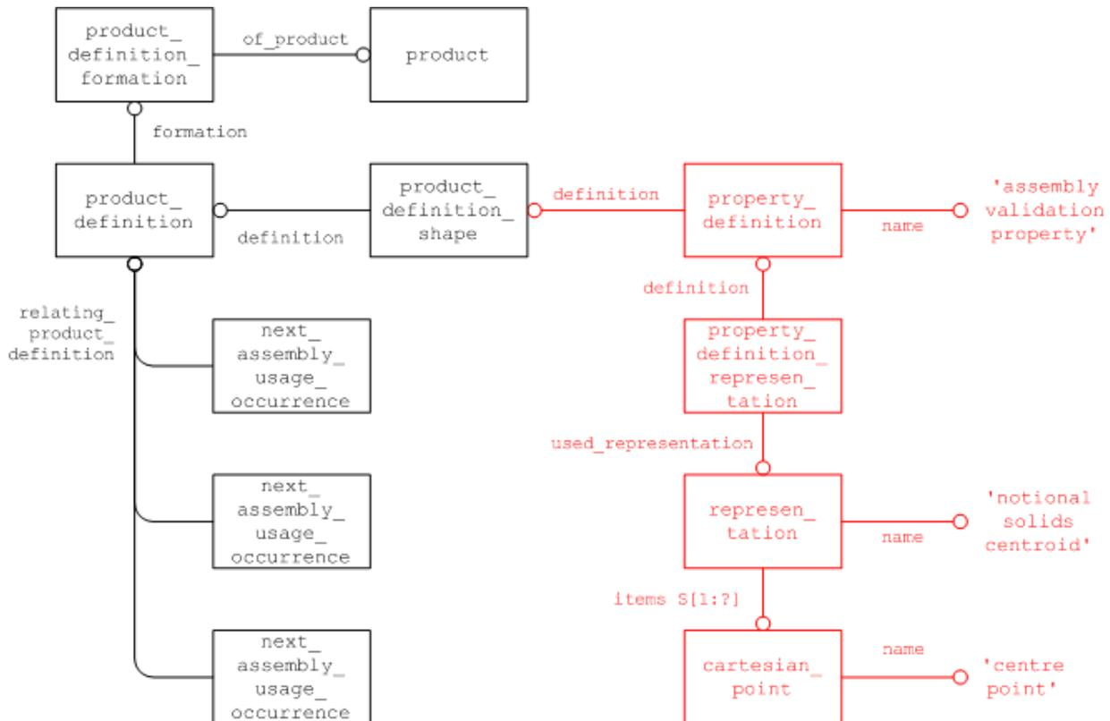
Figure 13: "Notional Solids Centroid Position" Validation Property
