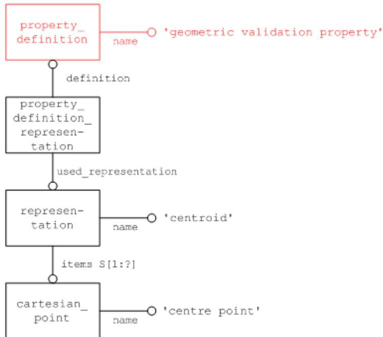
Figure 5: Geometric Validation Property "Centroid"
