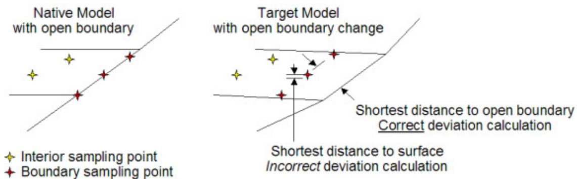
Figure 10: COPS - Sampling Points for an Open Boundary
