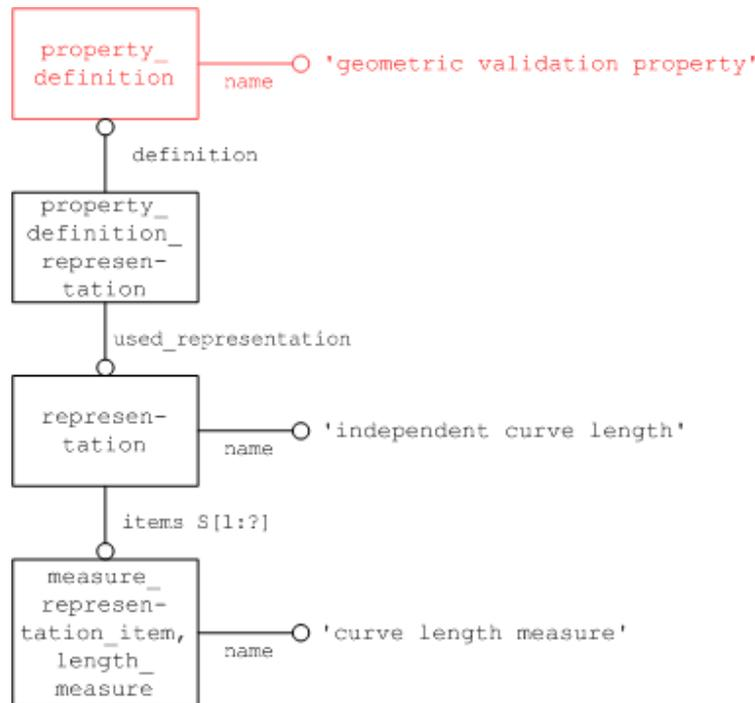
Figure 6: Geometric Validation Property "Independent Curve Length"
