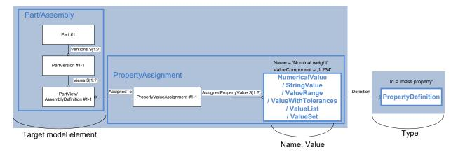
Figure 86: User defined attribute at the part/assembly level
