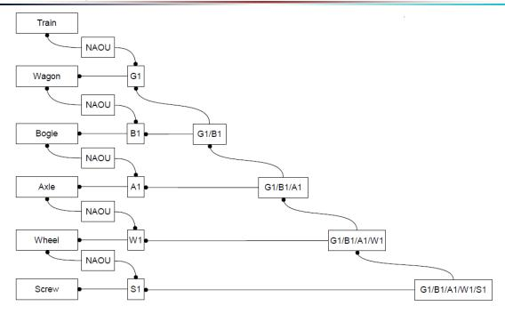
Figure 31: Instantiation without the intermediate SpecifiedOccurrences
