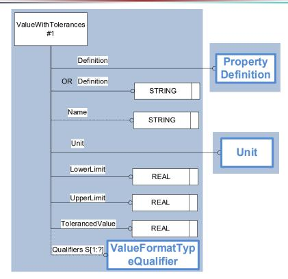
Figure 12: Template "ValueWithTolerances"
