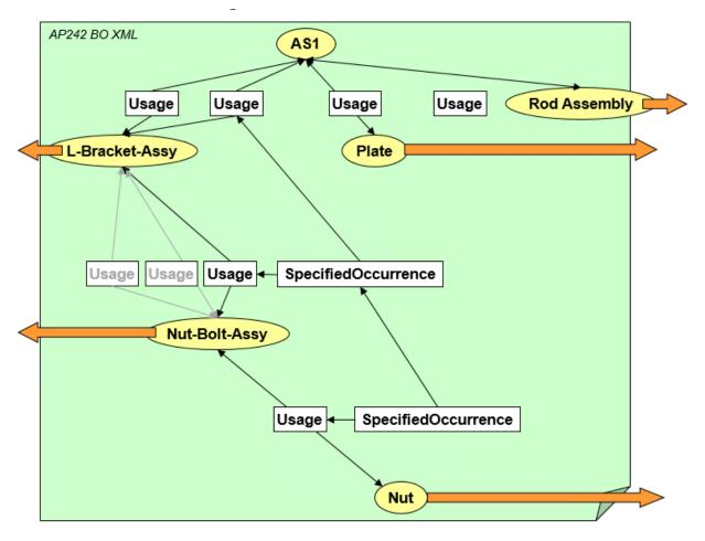
Figure 60: Example for Nested Structure with SpecifiedOccurrences
