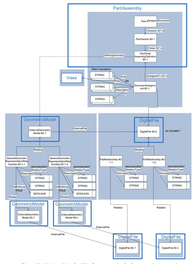
Figure 79: Model splitting for "CAx Representation for DocumentAssignment"
