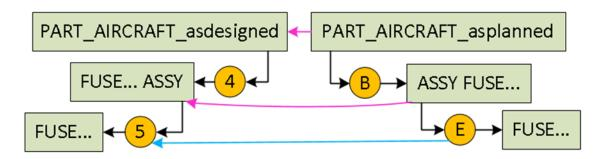
Here a valid example of PartView Relationships on level 1, 2 and 3, saying that all the occurrences of as-planned Fuse anywhere within the whole assy are tracked to the as-designed Fuse.
