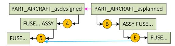
To do so, if the AsDesigned depth of the product structure is >1 and there is no tracking relationship defined on each parent level, the tracking relationships on the child levels shall reference SpecifiedOccurrences of the SingleOccurence on the parent level (see chapter 7.2):
