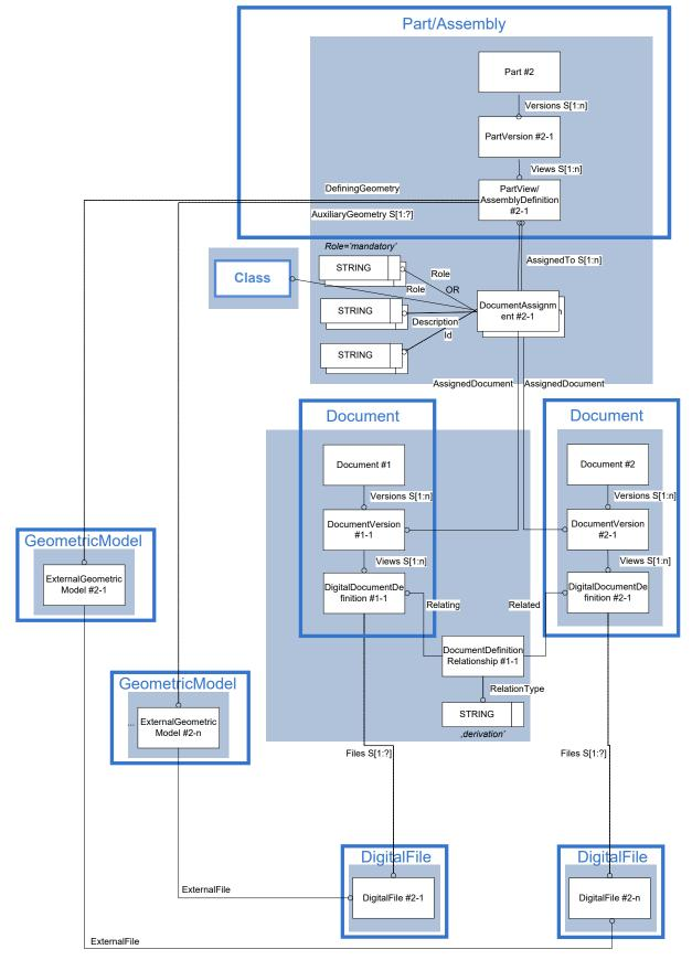
Figure 83: Alternate models for "PDM Representation for DocumentAssignment"
