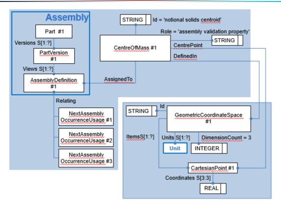
Figure 89: Instantiation of AVP 'notional solids centroid'
