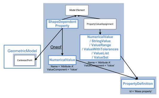
Figure 84: Definition of an attribute name and its usage
