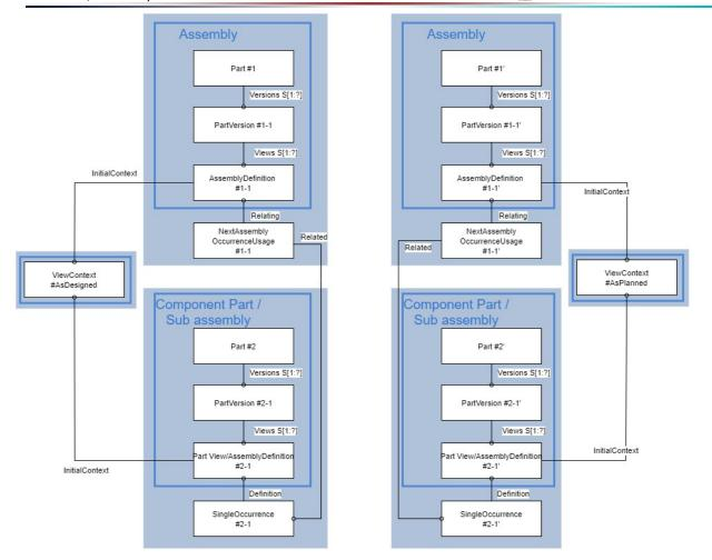
Figure 95: Representation of As Designed and As Planned views
