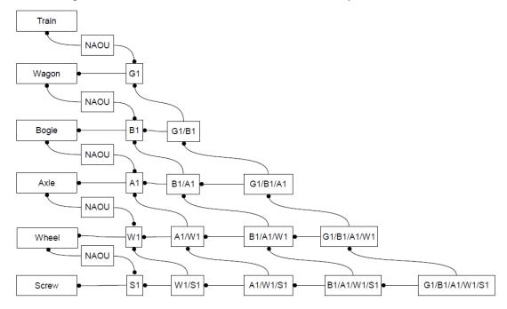
Figure 32: Instantiation with all the intermediate SpecifiedOccurrences
