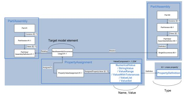
Figure 87: User defined attribute for a simple component instance in an assembly
