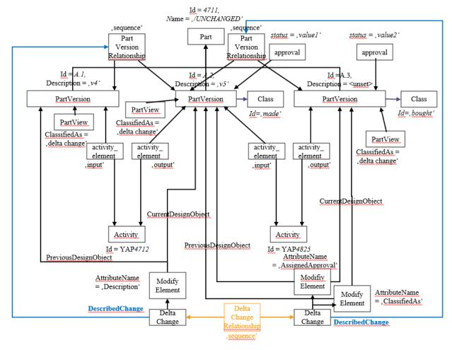
Figure 70: Example of a Delta Exchange for two sequential part changes which order is controlled between two DeltaChanges
