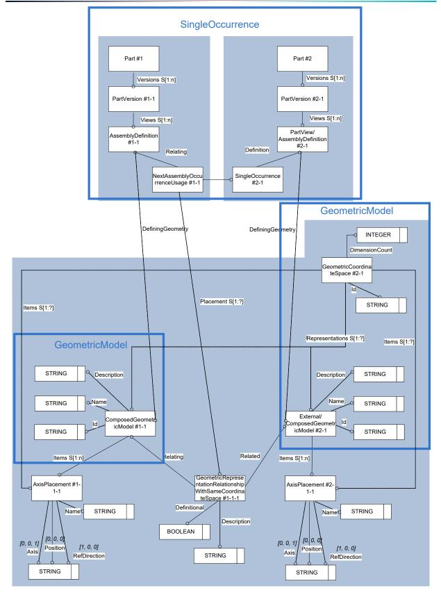
Figure 37: Full Positioning Representation with Same Coordinate Space
