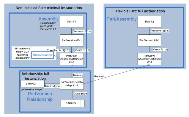
Figure 61: Special handling of additional 'Related' Parts after archiving/releasing the 'Relating' Part (here example of an additional shape as Flexible Part)
