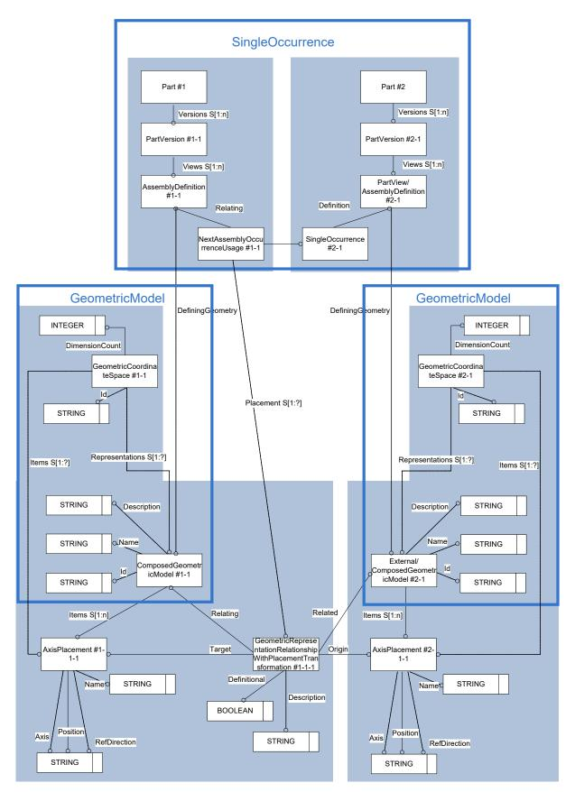
Figure 35: Full Positioning Representation with Implicit Transformation
