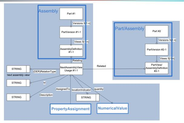
Figure 40: Template "PartViewRelationship" for quantity (+ properties)
