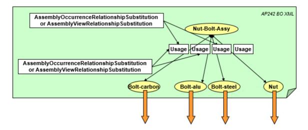
Figure 59: Example for Nested Structure with substitute parts
