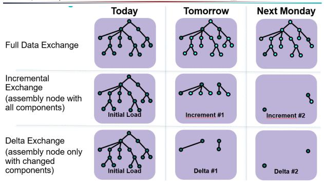
Figure 64: Differences between full data exchange, incremental exchange and delta exchange
