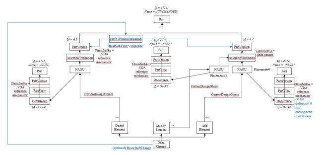
Figure 65: Example of a Delta Exchange on an assembly part with one component deleted, one added and one modified
