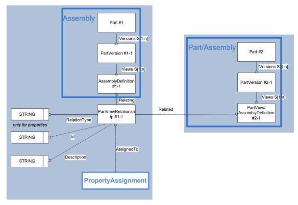
Figure 39: Template "PartViewRelationship" for properties
