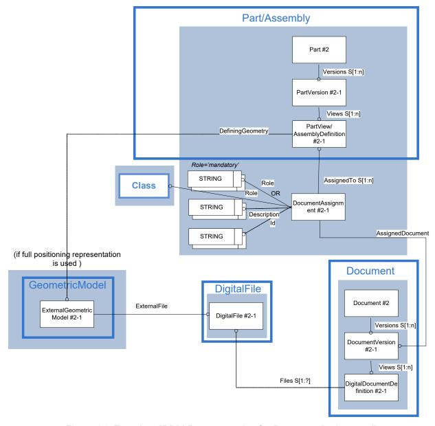
Figure 81: Template "PDM Representation for DocumentAssignment"
