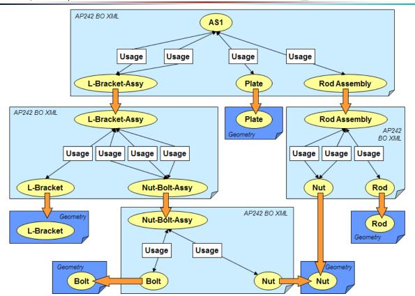
Figure 55: Example for not recommended Nested Structure
