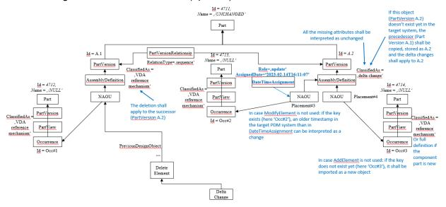
Figure 66: Example of the minimal instanciation of Delta Exchange of a new assembly version with one component deleted, one added and one modified
