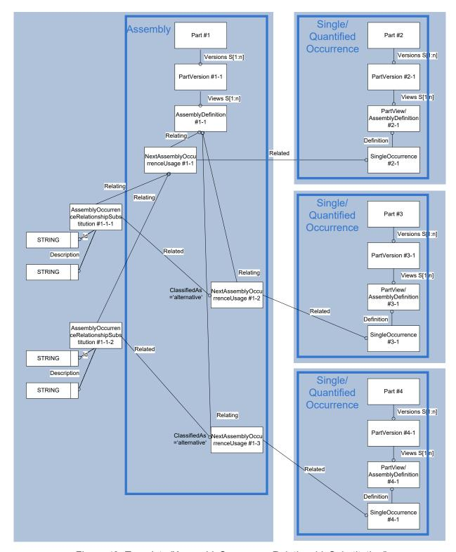
Figure 42: Template "AssemblyOccurrenceRelationshipSubstitution"
