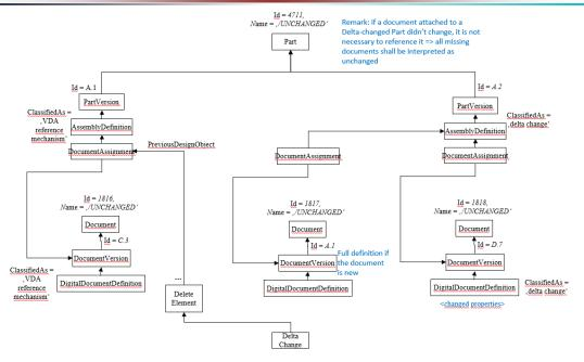
Figure 68: Example of the minimal instanciation of Delta Exchange of a new part version with one document deleted, one added and one modified
