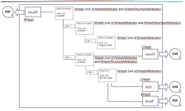
Figure 90: Example of LOTAR Product Structure Validation Properties at the single File, Part and Assembly level
