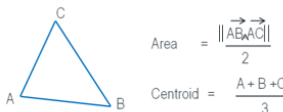
Figure 18: Calculation of Area and Centroid for a Facet
